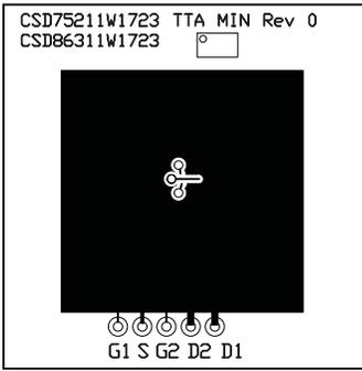
Max  $R_{\theta JA} = 68^{\circ}\text{C/W}$
